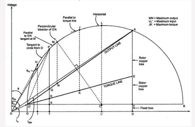
**Power scale**: As AD represents  $W_{SN}$  i.e. power input on short circuit at normal voltage, the power scale can be obtained as,
