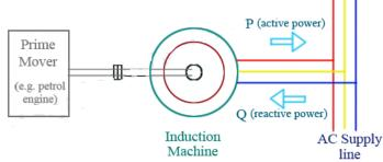
This generated rotor current produces a rotating magnetic field in the rotor which pushes (forces in opposite way) onto the stator field. This causes a stator voltage which pushes current flowing out of the stator winding against the applied voltage. Thus, the machine is now **working as an induction generator (asynchronous generator)**.
