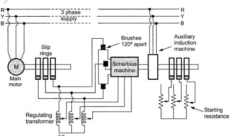
in the rotor of Scherbius machine, which is injected into the rotor of main motor. This controls the speed of the main motor.
