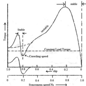
the torque developed by the motor may fall below this load torque. In this case, motor will not accelerate upto its normal speed, but it will run at a speed which is nearly 1/7th of its normal speed. This phenomenon is called as **crawling in induction motors.**
