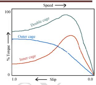
The torque speed characteristics of double squirrel cage motor for both the cages are shown in the figure.
