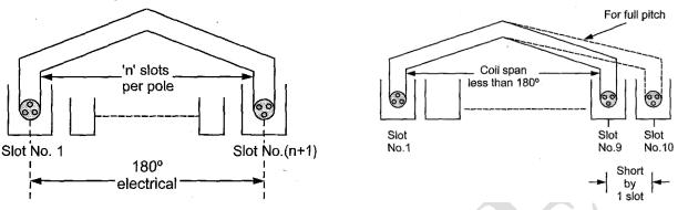
If coil span is slightly less than a pole pitch i.e. less than  $180^{\circ}$  electrical, the coils are called, short pitched coils or fractional pitched coils. Generally coils are shorted by one or two slots.
