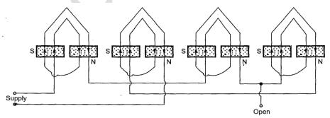
between this common point and the open third terminal, the poles are formed as shown in the Fig.
