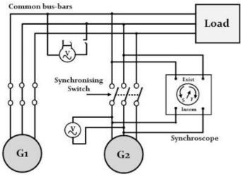
6. To match the terminal voltage of alternator-2 with bus-bar voltage we need to adjust the field current of alternator-2 until terminal voltage of alternator-2 matches with the bus-bar voltage. The required value of voltage can be seen in the voltmeter connected to bus-bar.
