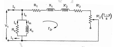
$R_{1e}$  = equivalent resistance referred to stator =  $R_1 + R_2$ '  $X_{1e}$  = Equivalent reactance referred to stator =  $X_1 + X_2$ '
