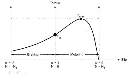
• Hence inspite of low braking torque, two lead connections is preferred over three lead connections. The torque-slip characteristic for motoring and braking operation is shown in the Fig.
