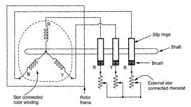
• In this type of rotor, the external resistances can be added with the help of brushes and slip ring arrangement, in series with each phase of the rotor winding.
