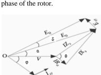
These components represent the  $I \cos \varphi$  and  $I \sin \varphi$  respectively. The power P converted internally is given be the sum of the product of corresponding components of the current with  $E \cos \alpha$  and  $E \sin \alpha$ .
