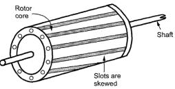
Skewing in rotor construction
