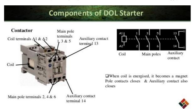
The contactor coil is connected in series with a start button, stop button and overload trip mechanism. This connection is called control circuit which is generally energized from two lines of three phase supply via a step down transformer.
