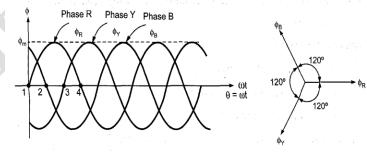
(a) Waveforms of three fluxes
