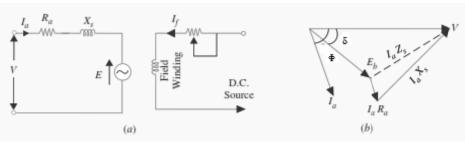
In other words,  $V = (-E_b + I_a Z_S)$ . The angle  $\delta$  between the phasor for V and  $E_b$  is called the load angle or power angle of the synchronous motor.
