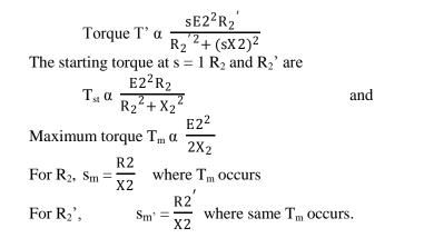
As  $R_2' > R_2$ , the slip  $s_m' > s_m$ . the starting torque  $T_{st}'$  for  $R_2'$  is more than  $T_{st}$  for  $R_2$ . Thus by controlling the rotor resistance the starting torque can be controlled. If resistance is further added to rotor, maximum torque is constant but slip at which it occurs increases and so starting torque increases.
