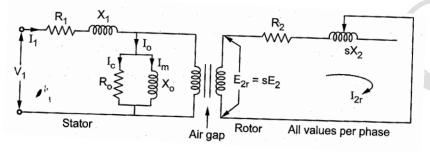
$I_{2r} = Rotor current per phase in running condition.$ =  $\frac{E2r}{Z2r} = \frac{sE2}{\sqrt{R2^2 + (sX2)^2}} A$ =  $\frac{E2}{\sqrt{(\frac{R2}{s})^2 + (X2)^2}}$
