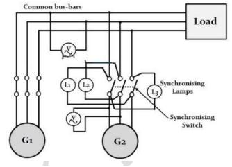
6. To match the terminal voltage of alternator-2 with bus-bar voltage we need to adjust the field current of alternator-2 until terminal voltage of alternator-2 matches with the bus-bar voltage. The required value of voltage can be seen in the voltmeter connected to bus-bar.
