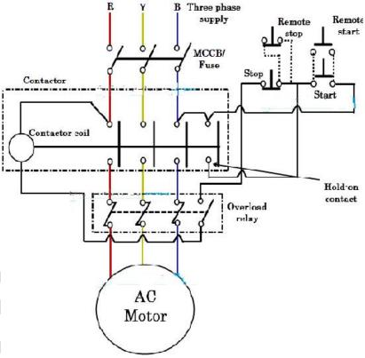
out the spring-loaded contact in the control circuit. The speed at which relay operates decided by the current adjustment. Typically it will be four to five times the rated motor current.
