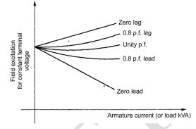
$\overline{E} = \overline{V}_t + \overline{I}_a (R_a + jX_s)$
