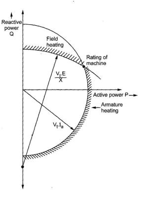
These two circles are represented in the Fig. The field heating and armature heating limitations on machine operation can be seen from this Fig. The rating of machine which consists of apparent power and power factor is specified as the point of intersection of these circles as shown in the Fig. So that the machine operates safely.
