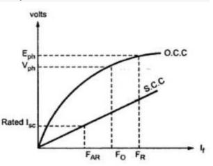
induced e.m.f.  $E_{ph}$ , required to get rated terminal voltage  $V_{ph}$ . This is possible from open circuit characteristics drawn. Once  $E_{ph}$  is known then the regulation can be obtained as,
