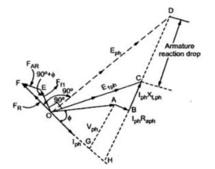
Once the total excitation is known which is  $F_R$ , the corresponding induced e.m.f.  $E_{ph}$  can be obtained from O.C.C. This  $E_{ph}$  lags  $F_R$  by 90°. The length CD represents voltage drop due to the armature reaction. Drawing perpendicular from A and B on current phasor meeting at points G and H respectively, we get triangle OHC as right angle triangle. Hence  $E_{1ph}$  can be determined analytically also.
