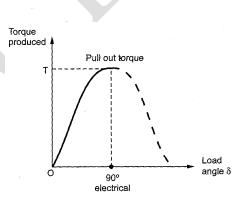
the synchronous speed. The amount of torque developed by the motor at the time of pulling into synchronism is called pull in torque.
