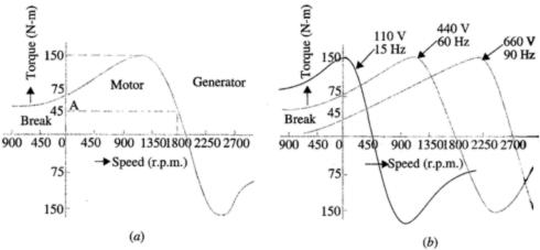
(speed axis) shifts with frequency. Since the shape of the torque/speed curve remains the same at all frequencies, it follows that torque developed by a SCIM is the same whenever slip speed is the same.
