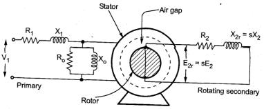
$X_{2r}$  = Rotor reactance per phase in running condition
