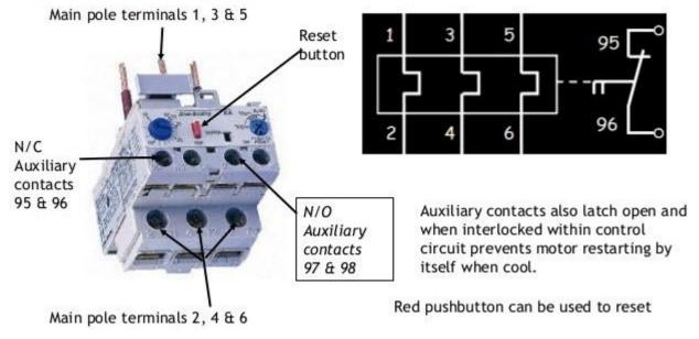
This overload mechanism should operate at 20 to 30% overload. When the overload coils trips, the current through the contactor coil stops flowing and hence the contactor contacts come to the OFF position. Overload relays are provided with current adjuster such that tripping coil current can be adjusted depending on the load protection requirement.
